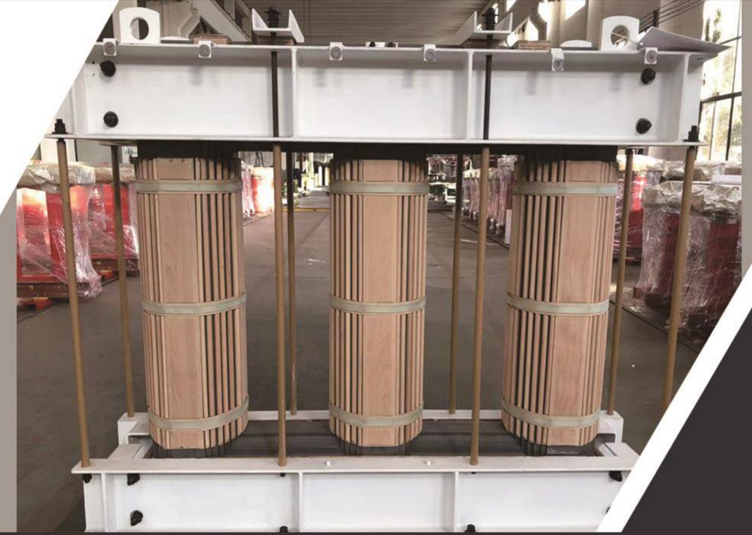
▲ 油浸接地变压器铁芯 Oil immersed grounding transformer core
