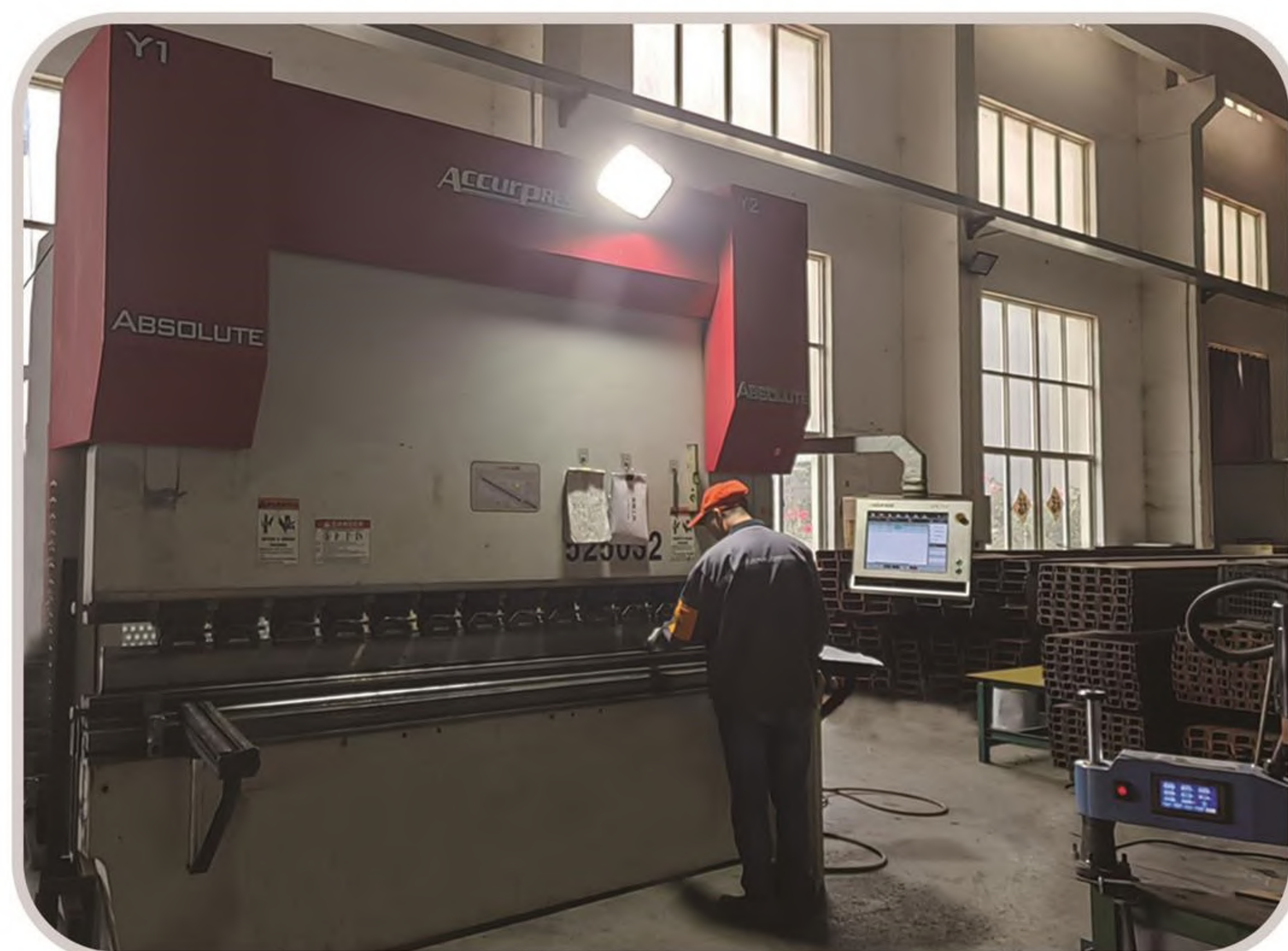
▲ 数控电液伺服折弯机 CNC ELECTRO-HYDRAULIC SERVO bending machine
