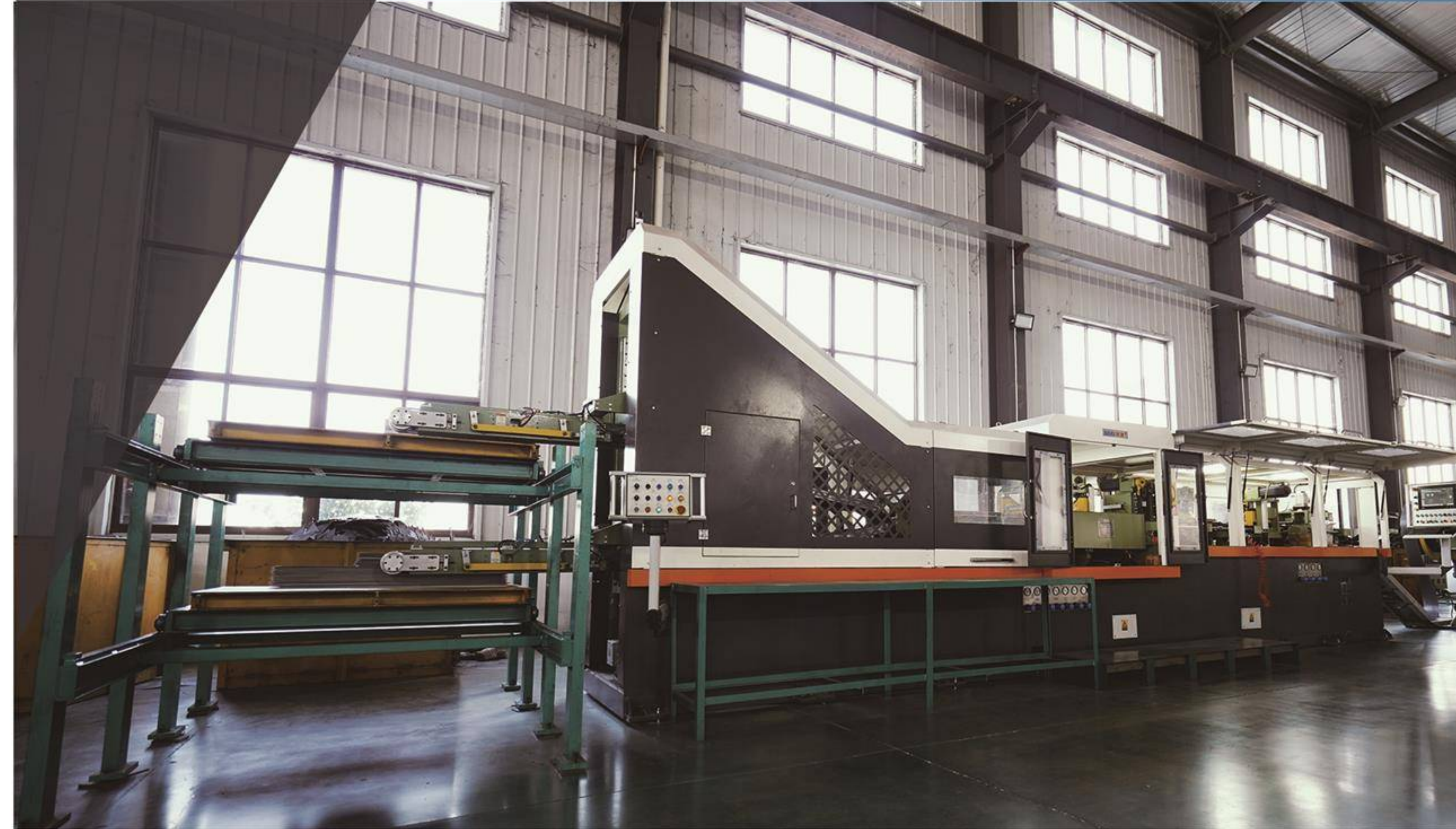
▲ 横剪线: 电动HJX (22) -400型 cut-to-length line: Electric HJX (22) -400
