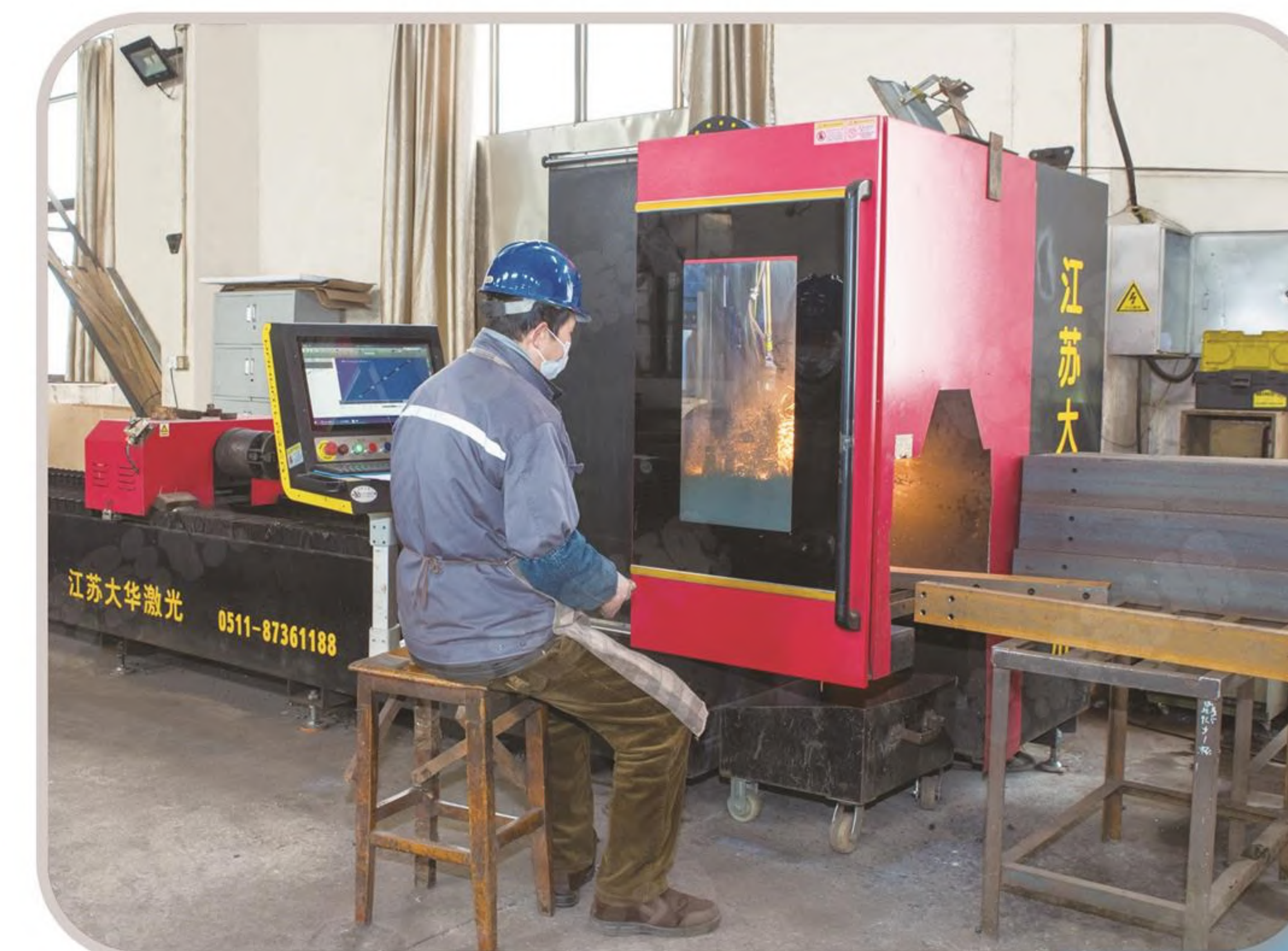
▲ 电纤激光切割机 Electric Fiber laser cutting machine
